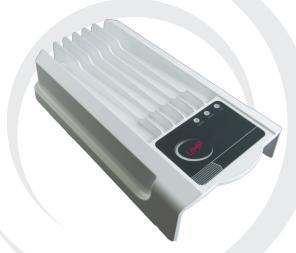
Multiple demodulators allow simultaneous reception of two TDM or SCPC carriers and group of TDMA mesh carriers. Universal modulator can instantaneously switch from TDMA burst mode to SCPC mode, thus assuring high data throughout and efficiency.
